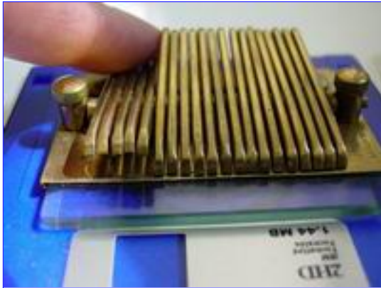
Photo 9. Weigl's clamp with 20 spring-loaded holders (clamps) which permit to immobilize 20 individual lice.
