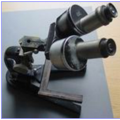
Photo 10. Low-power binocular magnifier (microscope) for facilitating the lice injecting and resecting
